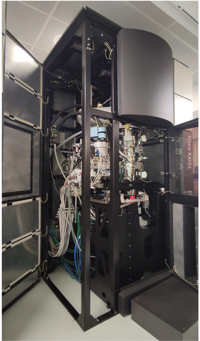
A. A modern dedicated cryo-TEM. B. The covers have been removed to show typical TEM features, such as the microscope column. The covers help in isolating the microscope from the environment to give stability while imaging. Image courtesy of Hari Venugopal, Monash University.
